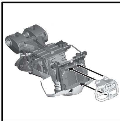
Turn the vehicle over. Fit the brush guard to the front end of the vehicle.
