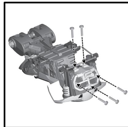
Insert five M4,5 x 1,9 cm screws into the brush guard and tighten.
